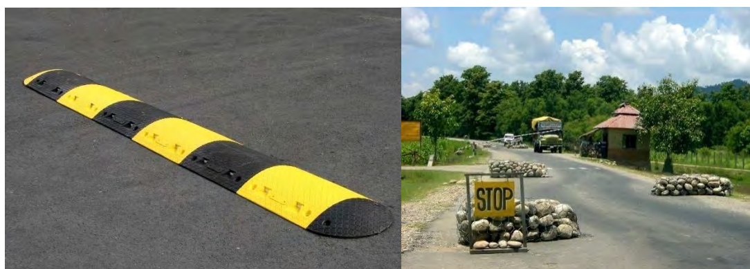
Figure 17: Traffic Calming Using: Speed Bump (left), Obstacles (Right)
